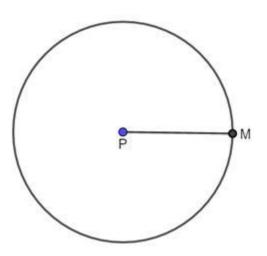
**iii.** Draw AB  $\perp$  PM such that AB passes through M, AB is required tangent.
