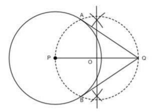
Q. 7. Draw a circle with radius 4.1 cm. Construct tangents to the circle from a point at a distance 7.3 cm from the centre.
